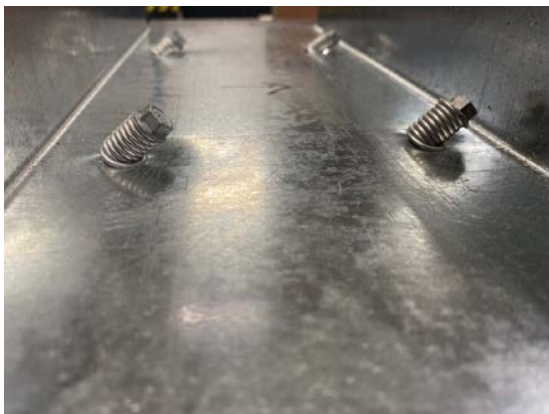
Figure 8-3: Test results - failure modes: Without spring wood failure (top); with without spring CFS track failure (middle); with compressed springs (bottom)
