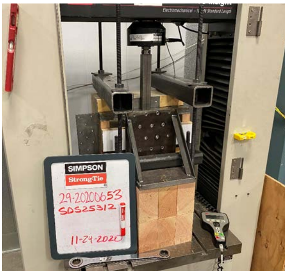
Figure 8-2: Test setup: Photo (left), schematic representation without gap (right top), schematic representation with 1/4" gap (right bottom)
