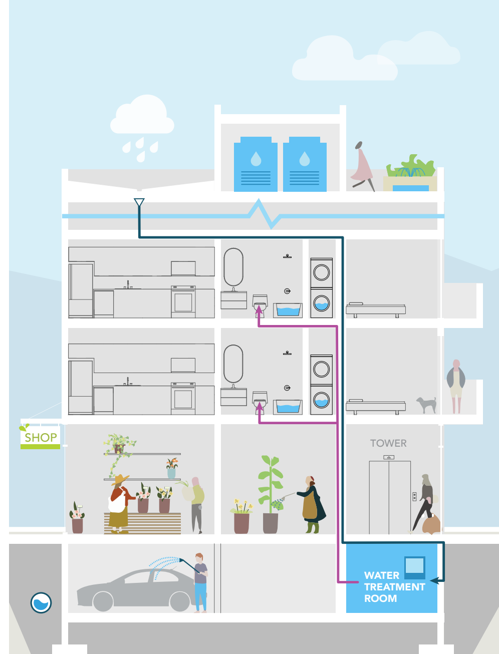
Figure 3: Buildings containing a non-potable water system require additional floorspace for water storage and treatment. Gross floor area exclusions can support various resilience measures.
