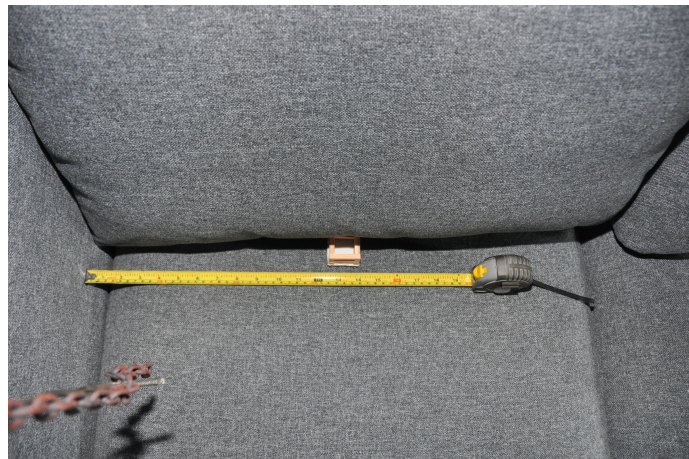
Figure 4: Position of the ignition crib on a couch cushion.
