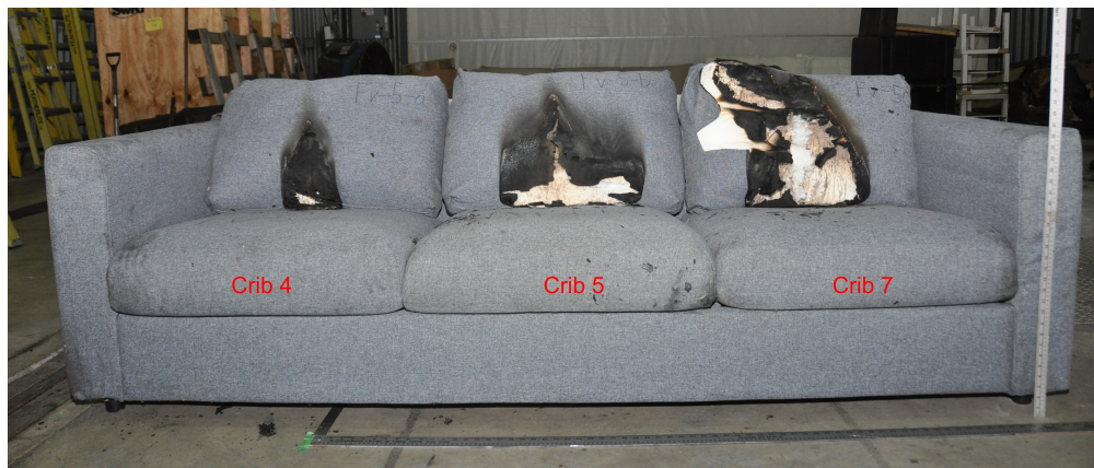
Figure 34: Front view of the FV5 couch showing burn patterns for each igniter crib.
