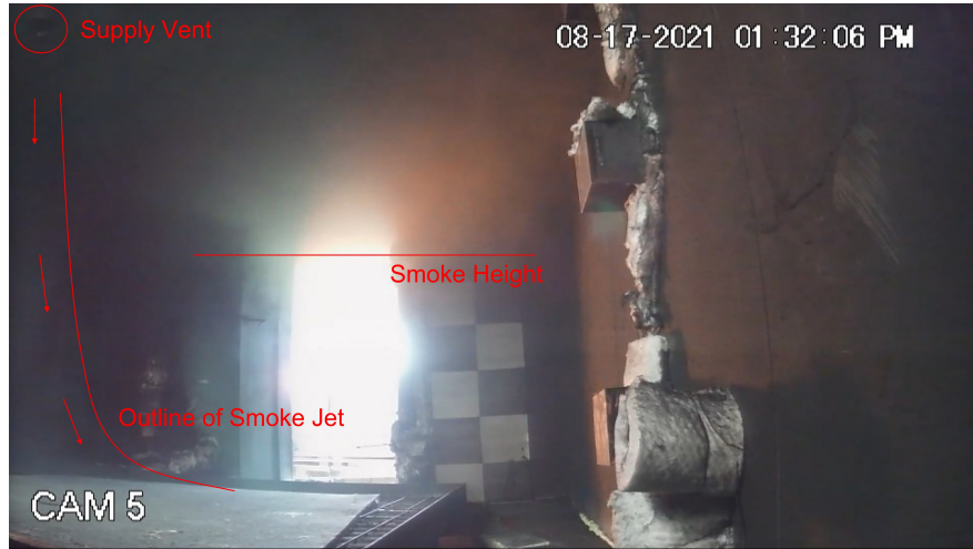
Figure 24: Images of smoke flow out of the first floor SW room supply duct in Test MV3.
