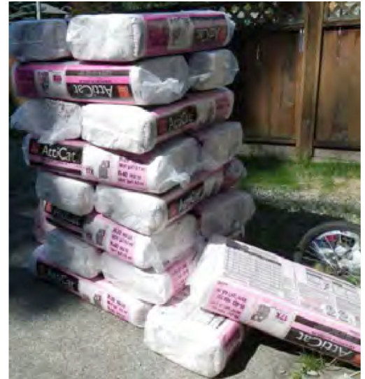
Blown-in insulation in packaging
