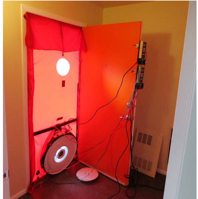
Typical blower door system installed in door frame for whole building airtightness testing.
