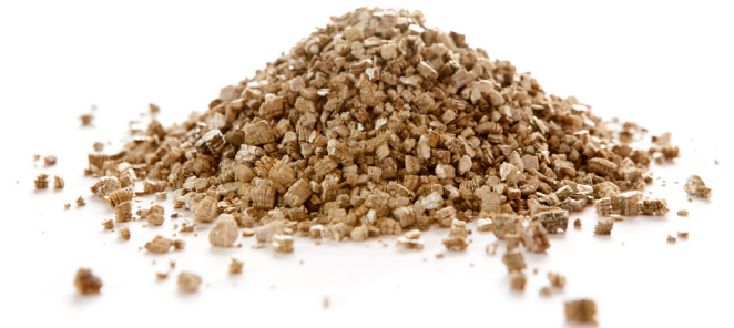
Vermiculite attic insulation potentially containing asbestos fibres.
