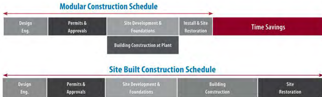
Figure 5: Modular Construction Timeline
