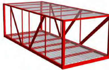
Figure 33: Fabrication Phasing on B2 BKLYN: World's Largest Pre-fabricated Building
