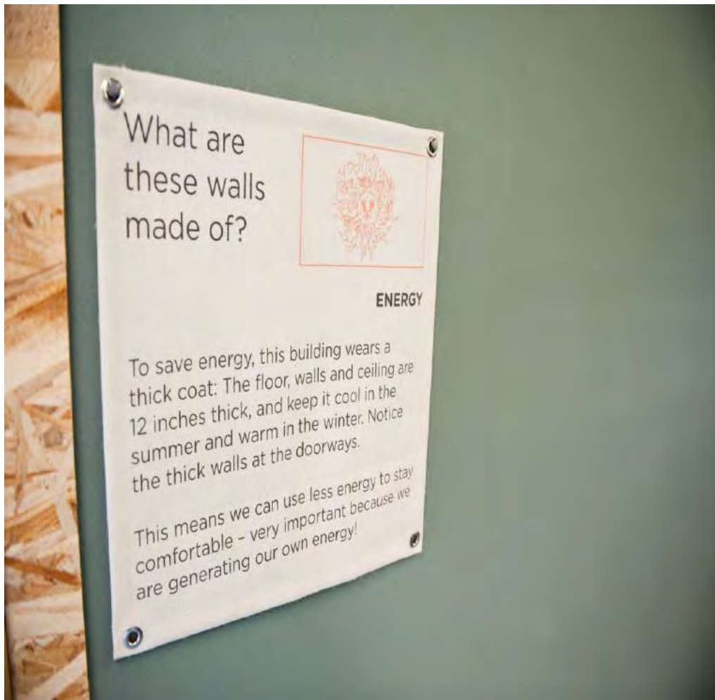
Figure 8: What are these walls made of? SIPs
